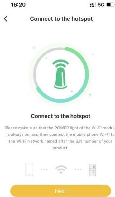
2. Step 1: Make sure the Power light on the WiFi module is always on and your phone is connected to the hotspot with the name of SN number.
